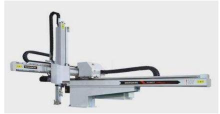
**BRB800~1200** Series is applicable to all types of horizontal injection machine ranges of 100~650T for take-out products and sprues. Vertical arm is telescopic type, suitable for two plate mold products take out. Traverse axis and vertical axis driven by AC servo motor. After installed this robot, the productivity will be increased 10~30%, reduce defective rate, ensure safety of operators, reduce manpower and accurately control the output to reduce waste.
